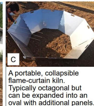
Figure 4.1. Schematic diagram explaining the principle of open-type portable flame-curtain kilns to produce biochar (adapted from Oo et al. 2018).
